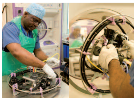
Easy loading: the dynamic oscillating load carrier allows operators to connect scopes away from the machine and has a simple lock-and-load mechanism
